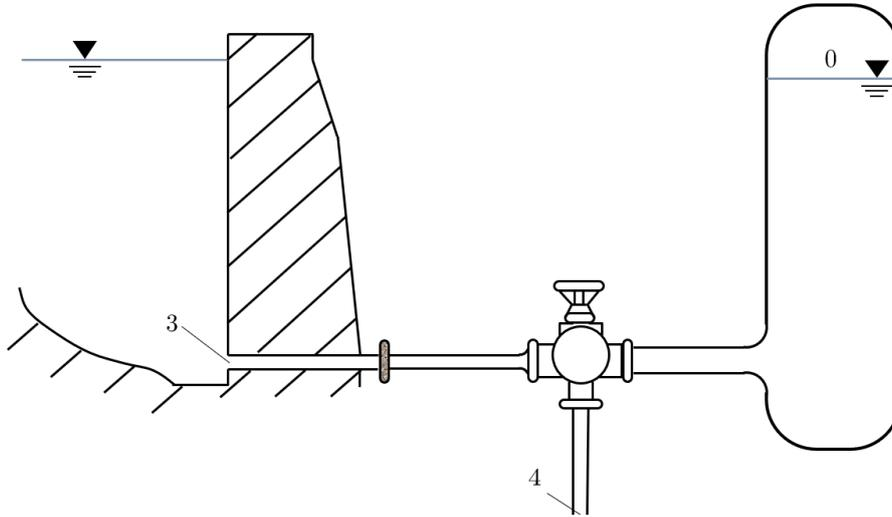
$$p_T + \rho g H = p_a + \rho g t + \frac{\rho}{2} v_3^2 + \frac{\rho}{2} v_3^2 \left( 2\lambda \frac{l}{d} + \zeta_S \right) + \frac{\rho}{2} v_1^2 \left( \zeta_V + \lambda \frac{l}{D} \right)$$
