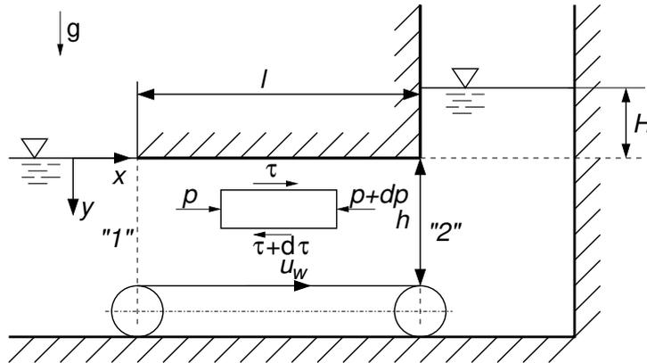
$$\left( p - \left( p + \frac{\partial p}{\partial x} dx \right) \right) dy + \left( \tau - \left( \tau + \frac{d\tau}{dy} dy \right) \right) dx = 0$$
